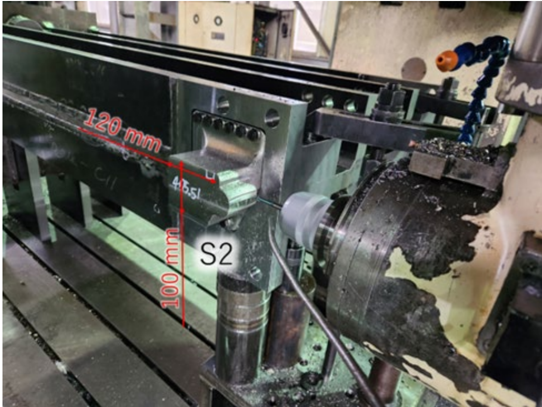
☒ 38 The final machining for S2 with the main body [26].
