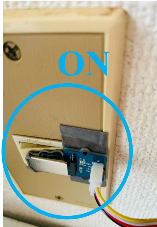
Figure 24. Bathroom Light Sensor (Light ON - Status1)
