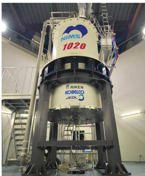
図 1-4 NMR 装置 (1.02 GHz)。K. Hayashi et al.: Journal of Magnetic Resonance, Vol. 256, pp. 30-33, 2015. 23) より引用。Copyright © 2015 Elsevier Inc. All rights reserved.
