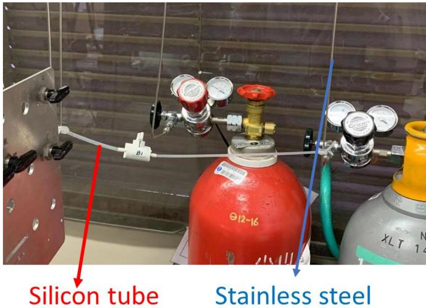
Fig. 3-12 Examples of silicon tubes and stainless steel pipes
