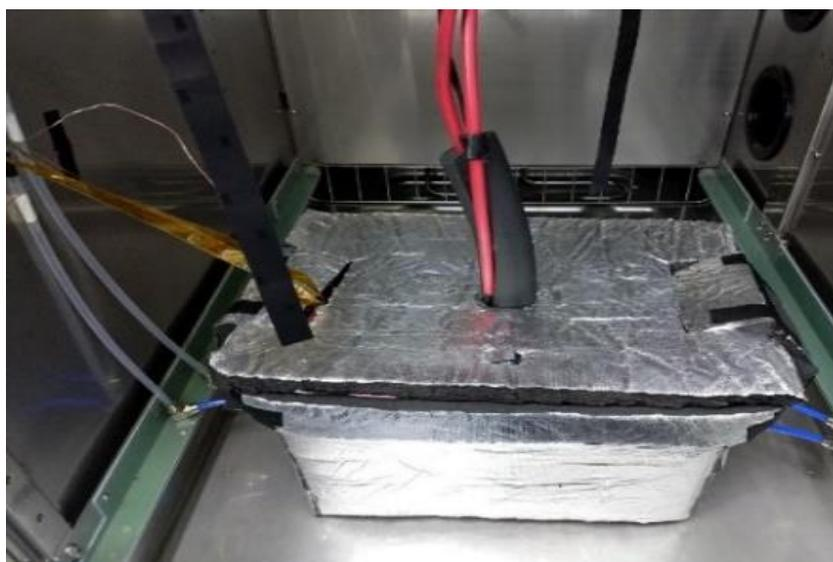
Fig.2-16 Box for heat insulation and heat insulation material around its perimeter
