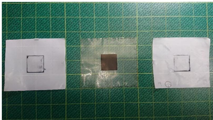
Fig. 3-10 The finished MEA after hot-pressing
