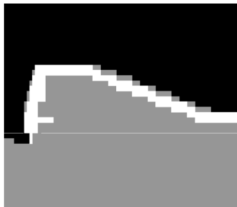
Figure 3.4. A simulated dike in CADMAS-SURF. The white color represents obstacles (impermeable structures); the gray color represents porous media; the white line represents the water level.
