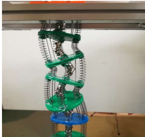
Fig.2-11. The buckling problem caused by too strong PtM springs hardness.
