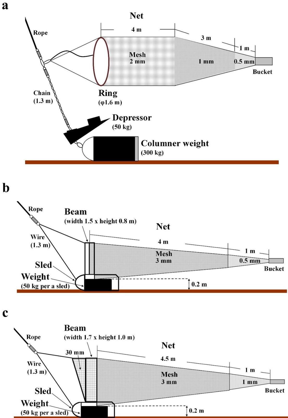
**Fig. 2** Schematic illustrations of collection gear. **a** ring net ( $\phi$  1.6 m); **b** beam trawl (wide 1.5 m  $\times$  height 0.8 m); **c** beam trawl (wide 1.7 m  $\times$  height 1.0 m)
