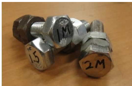
Figure 2-28 Three types of bolts to obtain the constant braking pressure (1 MPa, 1.5 MPa and 2 MPa)
