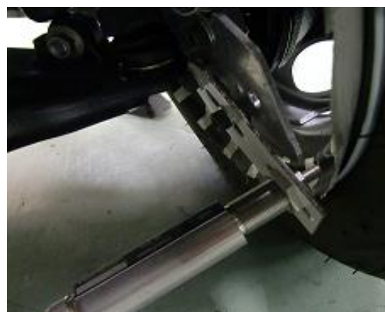
Figure 2-18 Photoelectric rotation detector at the rear tire (ONO SOKKI LG-916)
