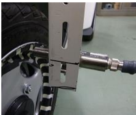
Figure 2-17 Photoelectric rotation detector at the front tire (ONO SOKKI LG-916)
