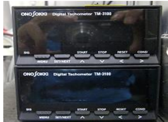
Figure 2-14 Digital display for rotation speed of the tire (ONO SOKKI TM-3130)
