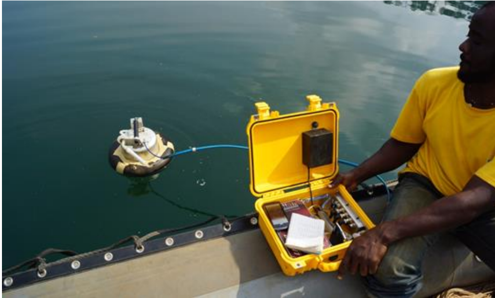
Photo III 1 CO 2 -flux measurement at water/air interface (Lake Barombi Mbo). The AC was adapted
