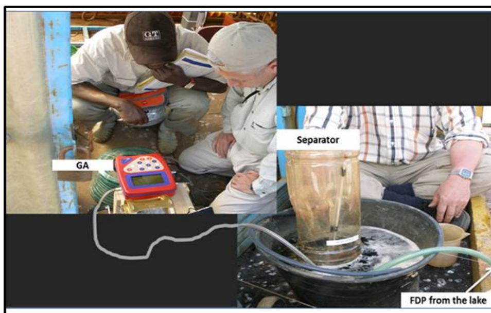
Photo III. 4 The GA is connected to the inverted separator to analyze the gas. Sampling and analysis of \text{CH}_4 and \text{CO}_2
