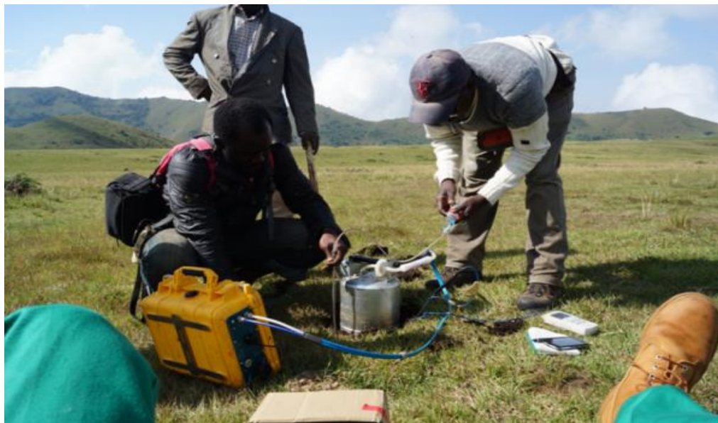
Photo III. 2 Soil CO 2 -flux measurement and gas sampling at Mt Manenguba Caldera
