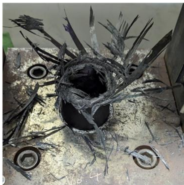
(a) Specimen C [45^\circ/0^\circ/-45^\circ/0^\circ/45^\circ]
