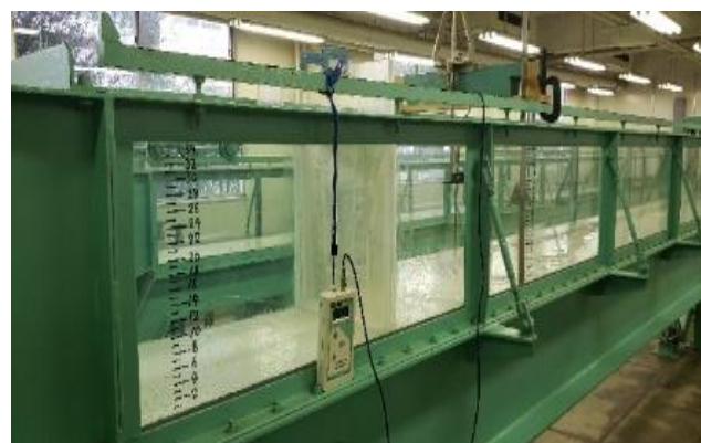
Fig. 7 Dam-break experiment in a rectangular channel.
