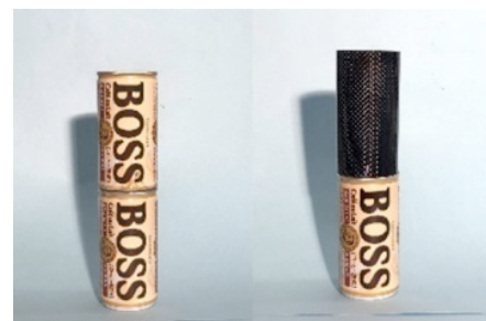
(a) Steel + Steel (b) CFRP 3Ply + Steel
