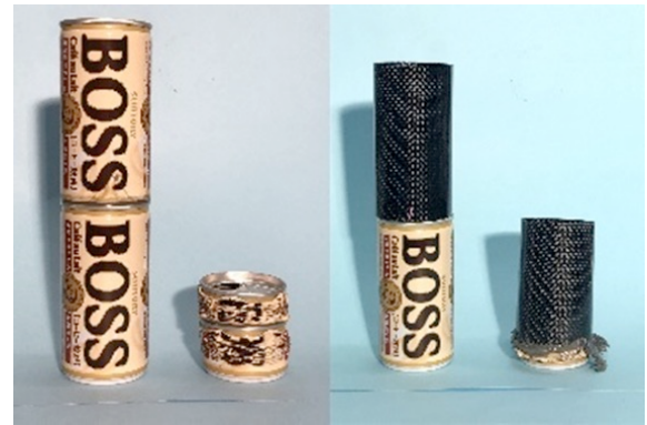
Fig. 6 Comparison of the test piece crushed in the drop weight test and the test pieces before the test.
