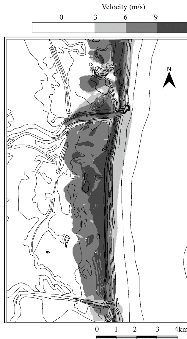
Fig. 6 Tsunami velocity after 28 minutes of the calculation start.
