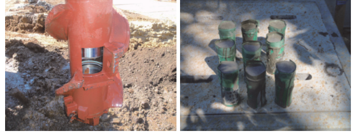
Fig. 2 Sampler and specimen of fresh soil-cement.
