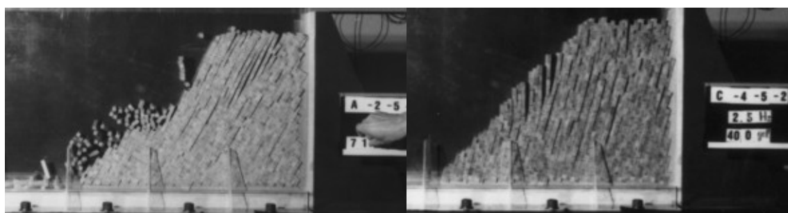
Figure 5. Several views of model tests on jointed rock slopes with a thoroughgoing discontinuity set during 1984–1986 at Kawamoto Laboratory of Nagoya University (Shimizu et al. , 1998; Aydan et al. 1989, 2006a, 2006b)
