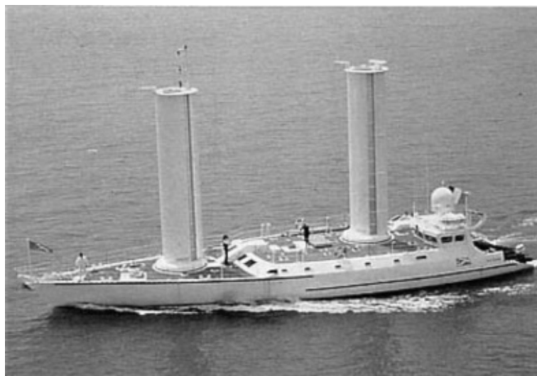
Alcyone launched in 1983 Photo 4 Alcyone equipped with twin turbo sail system.
