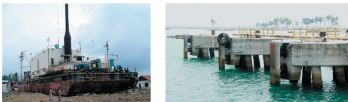
Figure 12 Displaced barge with a power generator and its wharf (JSCE, 2005)
